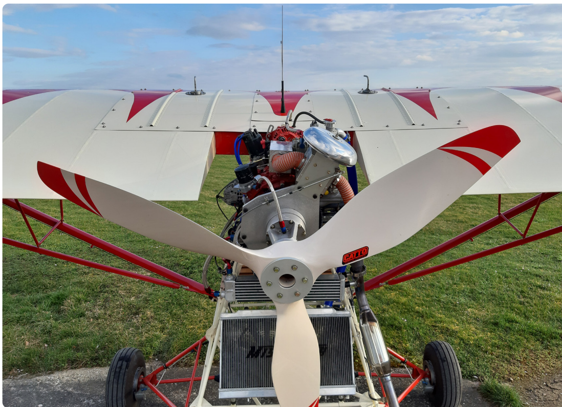
To power his Breezy, Carl-Friederich chose a modified Mazda 13B rotary engine and a custom Catto propeller.
